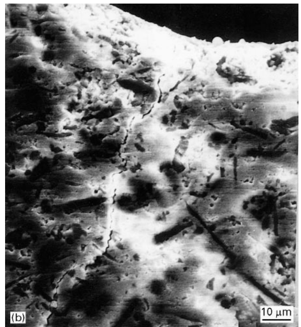
Figure 7 Scanning electron micrographs of the in situ tensile specimen of 20 vol % SiC w -ZrO 2 (2 mol % Y 2 O 3 ) composite, (a) before tension, (b) after tension showing the initiation of the crack at the notch.
