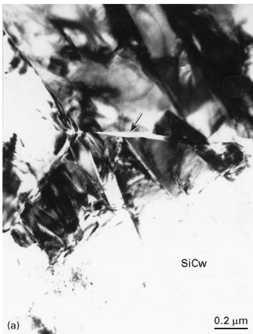
Figure 2 Transmission electron micrographs of the ZrO 2 matrix in 20 vol% SiC w -ZrO 2 (2 mol% Y 2 O 3 ) composite showing microcracks induced by t → m ZrO 2 transformation.
