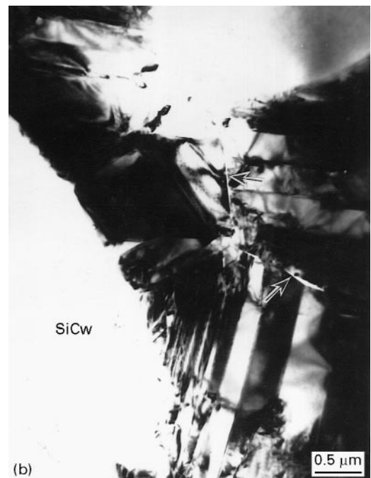
Figure 2 Transmission electron micrographs of the ZrO 2 matrix in 20 vol% SiC w -ZrO 2 (2 mol% Y 2 O 3 ) composite showing microcracks induced by t → m ZrO 2 transformation.
